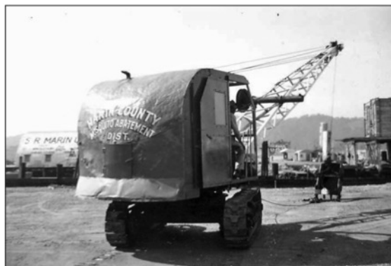
Motorized equipment greatly facilitated the District's operations, allowing ditches to be cleaned with equipment such as this dragline (pictured here at the District's premises).
