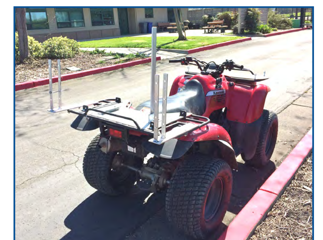
A vertical aluminum post on the rear plate provides the anchor for a backpack duster/blower unit.
