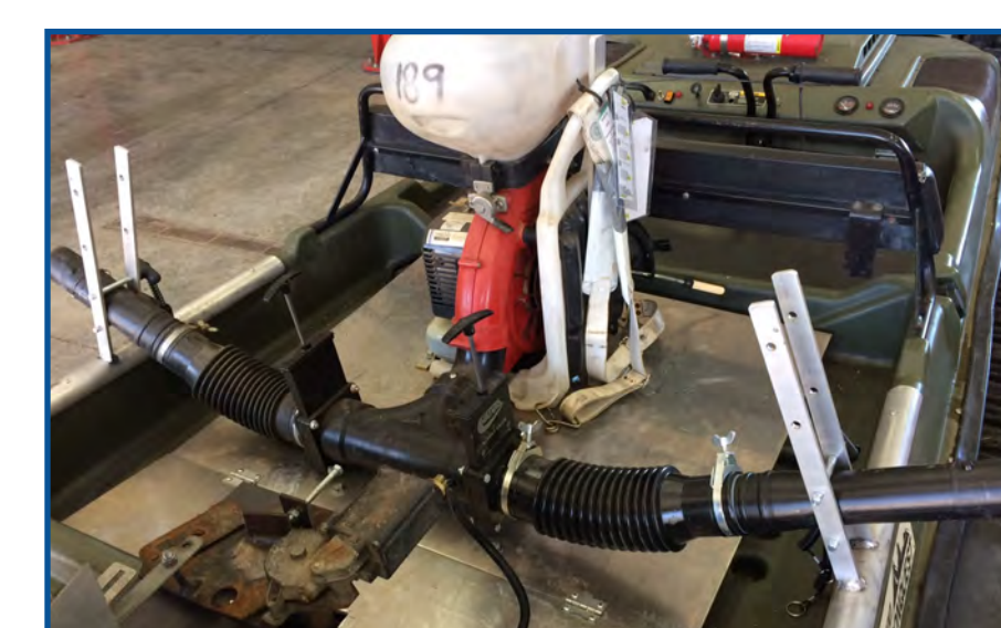
3" dual cleanout tee splits flow from blower; RV waste gate valves control flow to each hose.
