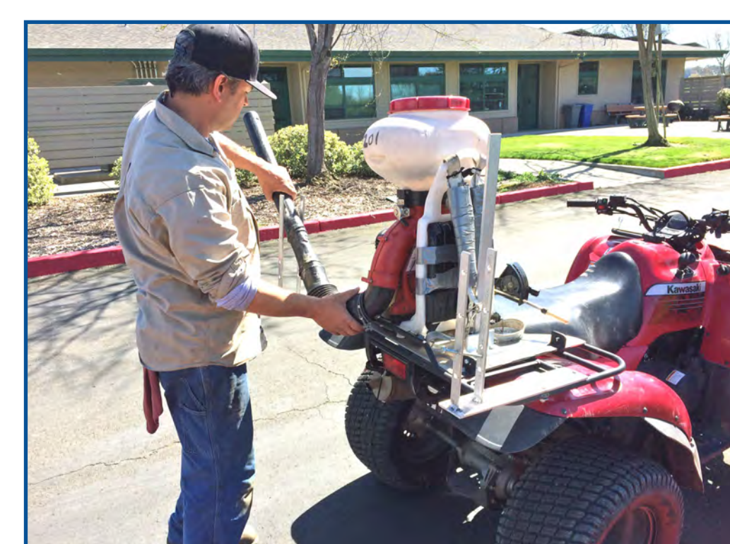
The duster/blower hose can be directed to face either side of ATV.
