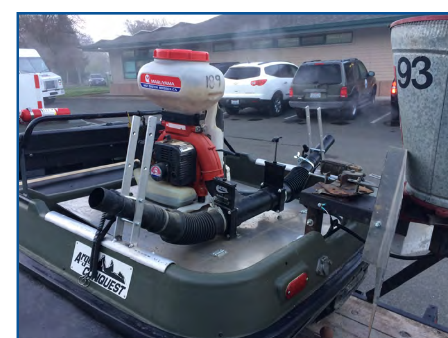
Duster/blower hoses (shown w/o extensions) lock into upright guides.
