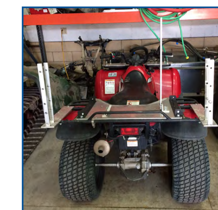
Rear equipment plate also includes brackets for mounting a spray tank.
