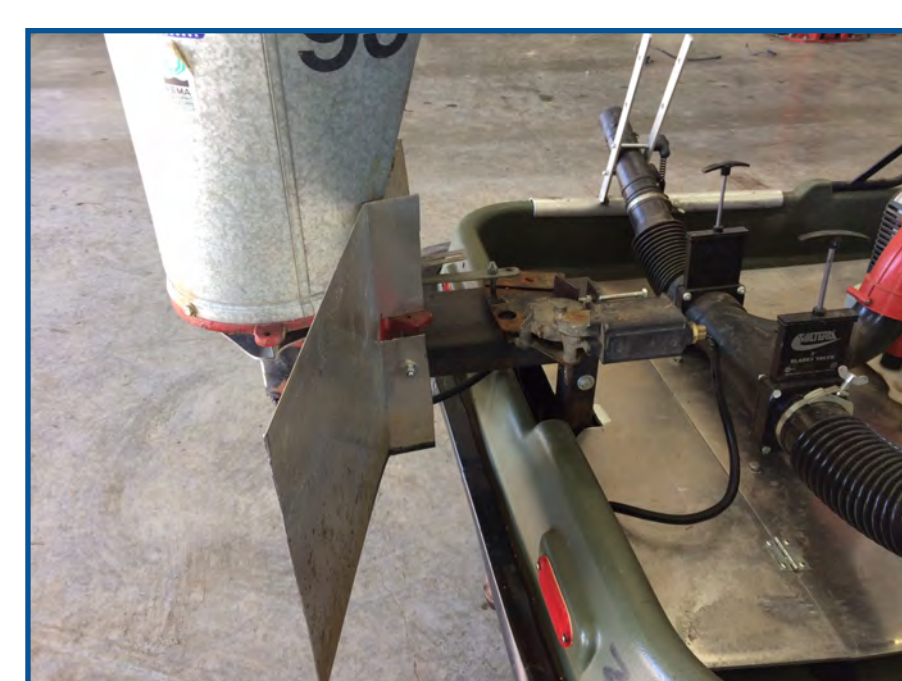
Removable sheet metal plates prevent blowback of material into vehicle.
