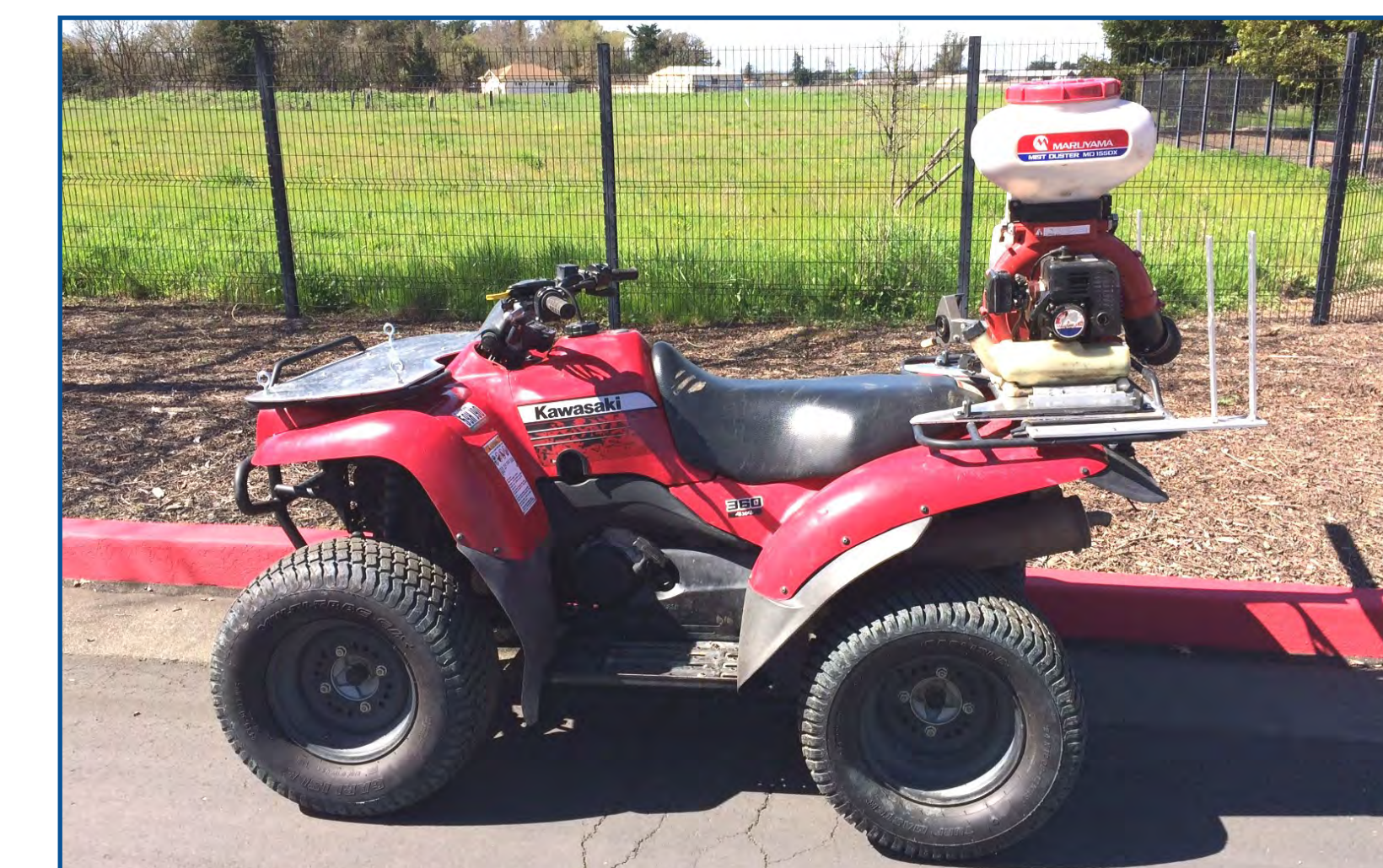
Lightweight 1/4" aluminum plates were mounted on the ATV. The front plate includes eye bolts to tie down bags of material or secure cargo basket.
