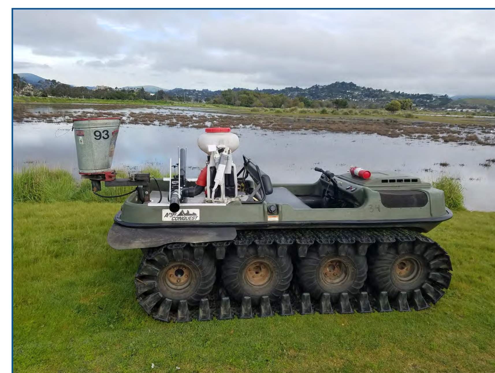
Combined application from duster/blower and rear-mounted seed broadcaster creates a 50' swath.
